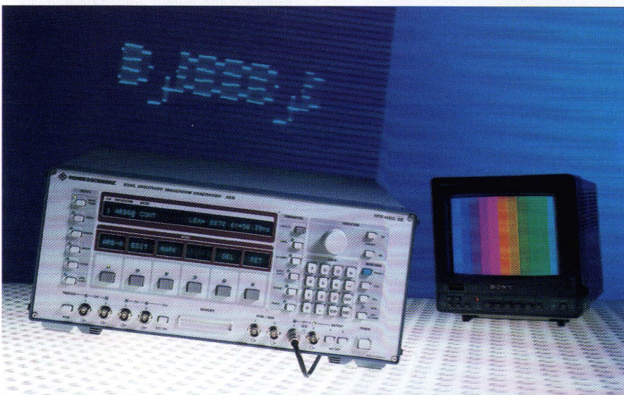
FIG 1 Arbitrary Waveform Generator ADS as signal source for generating colour-bar test patterns Photo 39 721
